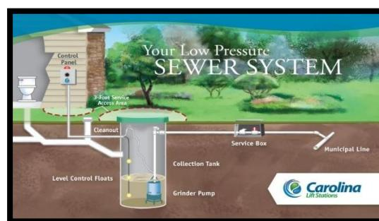
The above pictures are sample of what the system will be like. Each property will have a grinder pump unit that will pump liquid waste to the main collection line going to the wastewater treatment plant.
